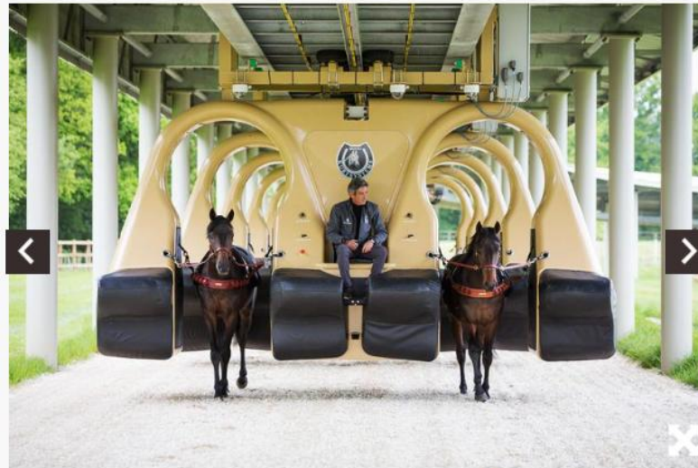
Kurtsystems' cabins can take up to 10 horses at varying speeds, from a trot to a canter, around the all-weather surface
